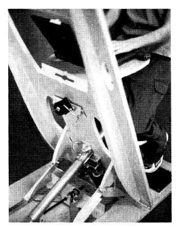
Fig. 2. The microcontroller and actuators of the Laptop Easel
