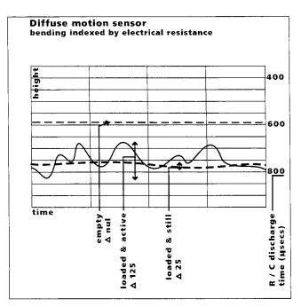
Fig. 7. Degrees and patterns of electrical activity due to bending.
