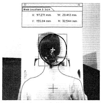
Fig. 8. Numerical data representing blob centers and blob extents is derived in hardware from the video stream, and sent to the microprocessor for the interpretation of posture.
