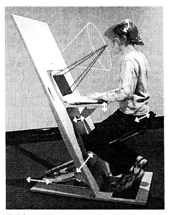
Fig. 3. Sensors and actuators watch and correct your posture while you concentrate on a different set of tasks.
